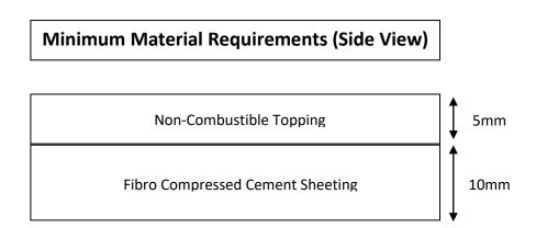
The hearth must be a minimum of 980 x 980mm for a square-on installation (front corners can also be cut as seen below).
